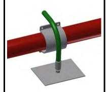
Hose assemblies must be protected against the effect of temperatures if these exceed the values given in the catalog. Particular attention should be paid to the laying of hose assemblies in the range of heat sources. Hose assemblies should be protected by protecting equipment such as protecting hose.
