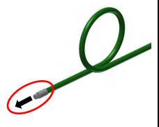
The development of hose loops must be avoided and counteracted. Tensile forces by pulling at those loops are also to be avoided.
