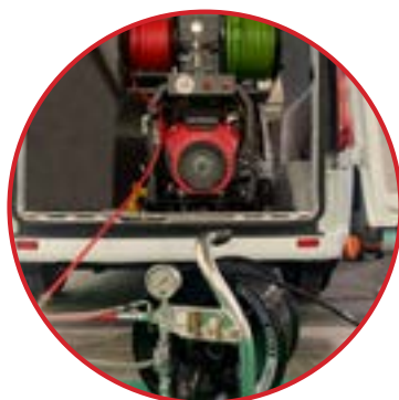
domestic drains and condominal sewer cleaning units
