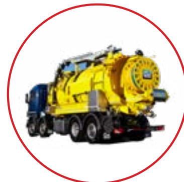
Vehicles equipped for water jetting
