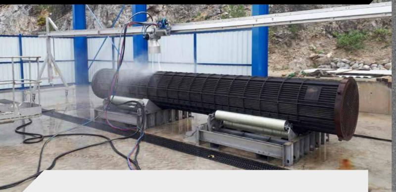
AUTOMATED SOLUTION FOR EXTERNAL CLEANING OF HEAT EXCHANGER TUBES
