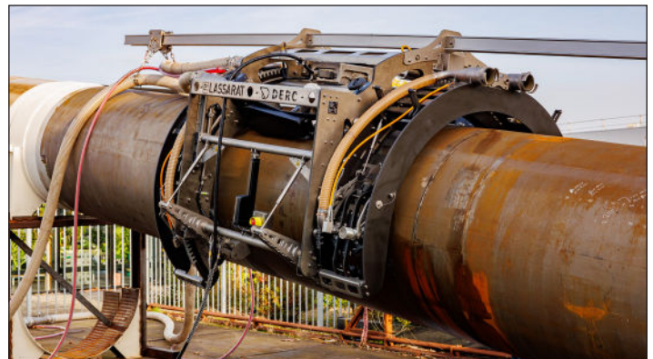
DERC XXL R-Tube innovative pipe-cleaning robot
